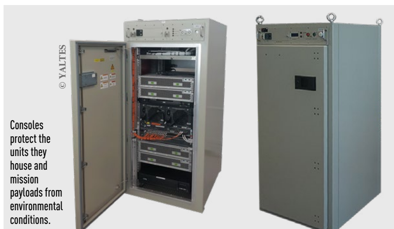
YALTES uses 30-inch displays in its new generation consoles. This allows the display to show images from radars or electro-optical sensors and mission management applications together.
